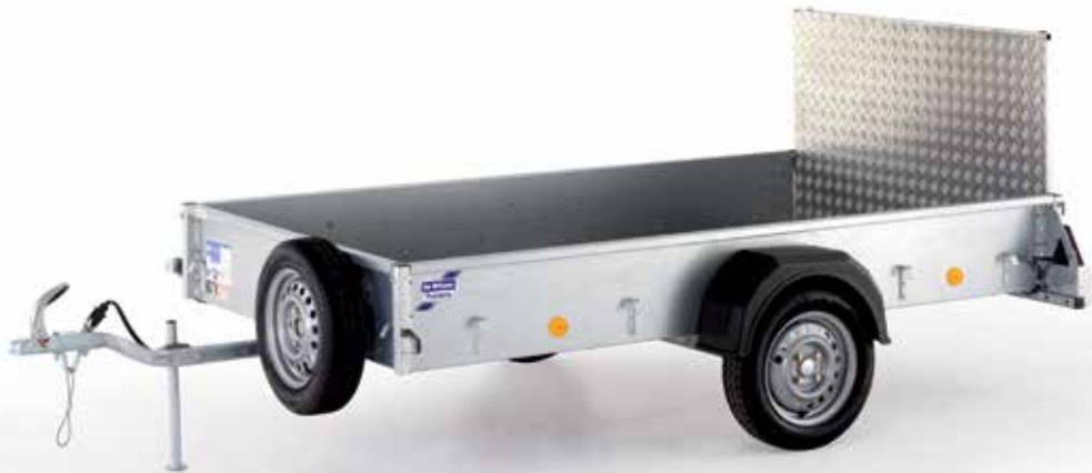
P8e trailer with ramp and 145/70R13 tyres
